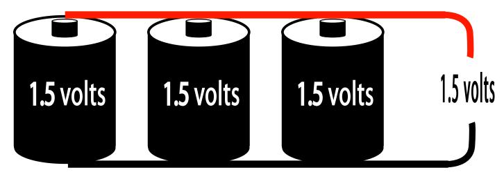
Capable of delivering amperage equal to that of 3 individual cells
