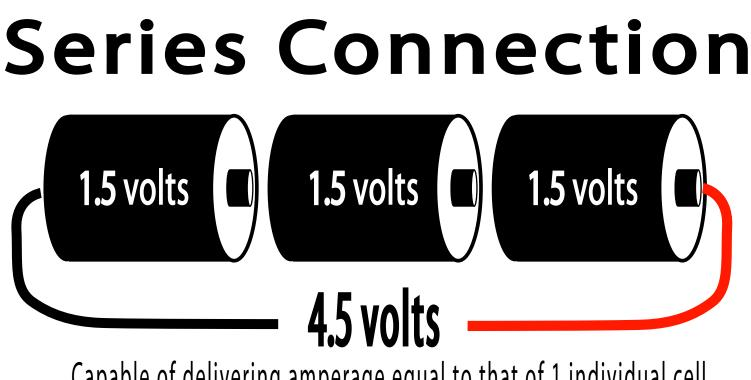
Capable of delivering amperage equal to that of 1 individual cell
