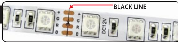
If you have purchased a strip longer than 2", you may cut those strips at any of the black lines like the one shown in the image. Make sure to cut in the middle of the contact terminals to allow enough space on each strip to attach wires.
