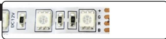
Locate the contact points at the end of your strip. These contact points are where you will solder in order to connect your light strip to your 4-pin connector (#LED-RGBCON-1). There are four (4) contact points and they are labeled + (positive), G (green), R (red) and B (blue).
